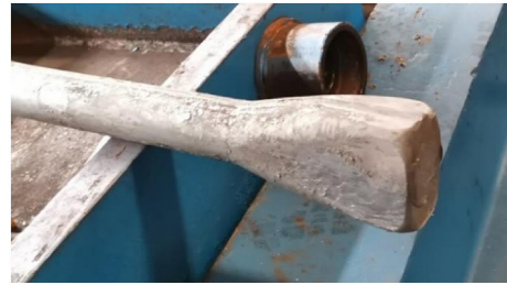
图 15 第 3 道次墩粗聚料后的产品 Fig.15 Product after the third rough upsetting
